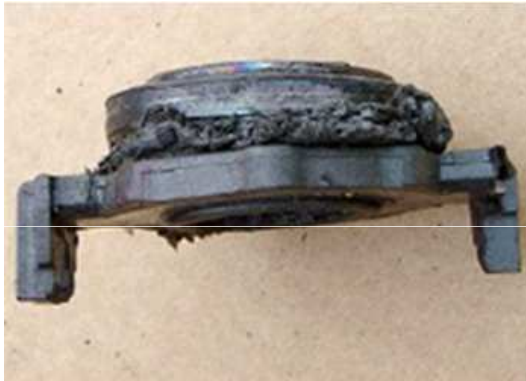
Bearing overheating further to a lack of preload
