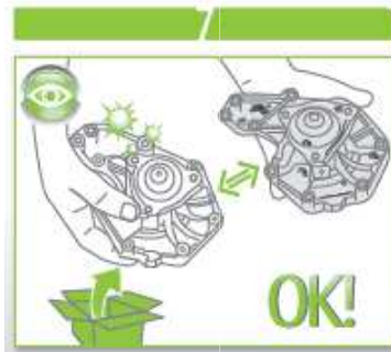
Step 7: Check the new water pump
