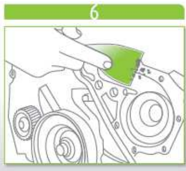
Step 6: Clean the engine surface
